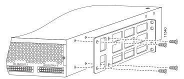
Note: The second bracket attaches to the other side of the chassis.
